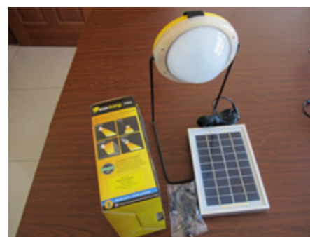
SunKing Pro (Greenlight Planet) with 2.5 Wp plug-in PV module (so that light does not have to be left out in the sun to charge up), variable brightness settings and an integrated phone charger.
